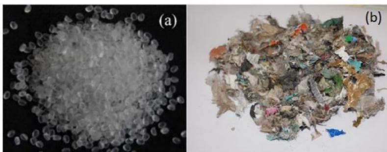
Fig. 1. Example of conventional (a) vs non-conventional (b) plastic solids.
